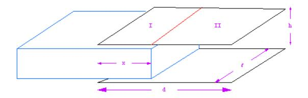
35. Consider a rectangular piece of dielectric that fills the space between the plates, partially inserted into a plane – parallel condensor. What are the energies of the system as a function of position, and hence the forces
