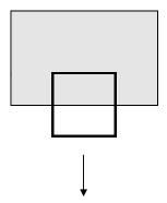
Calculate the terminal velocity of this loop, in meters/second, given B = 1 Tesla, the resistivity of Aluminum =  $2.65 \times 10^{-8} \Omega \cdot m$ , and  $g = 9.8 m/s^2$ .
